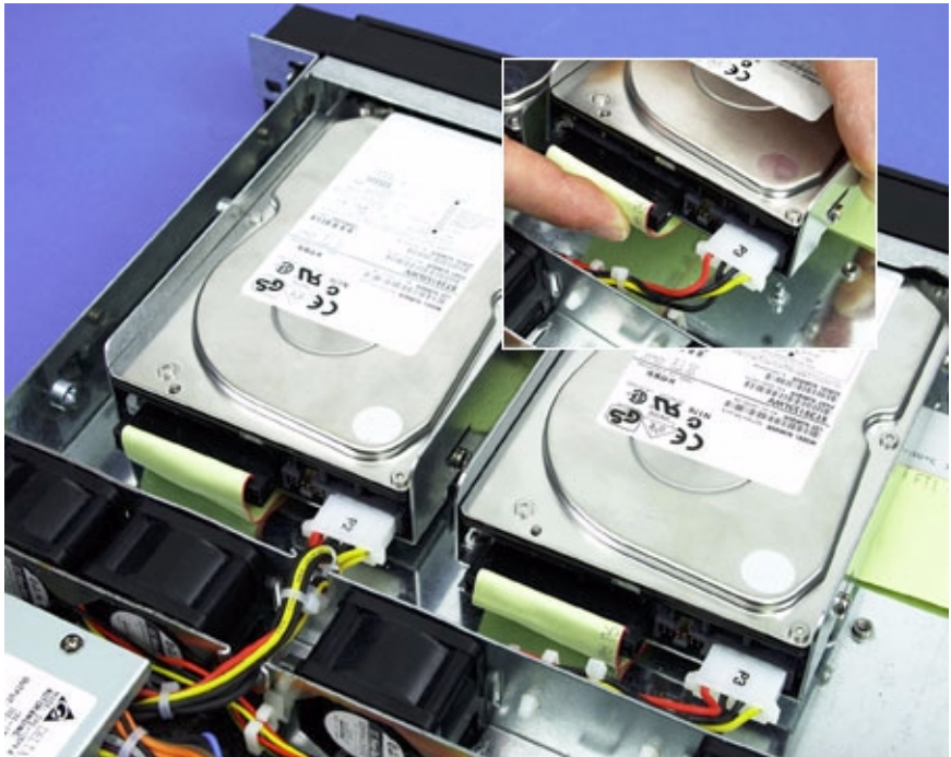
Figure 14 Drive Bay Installation
